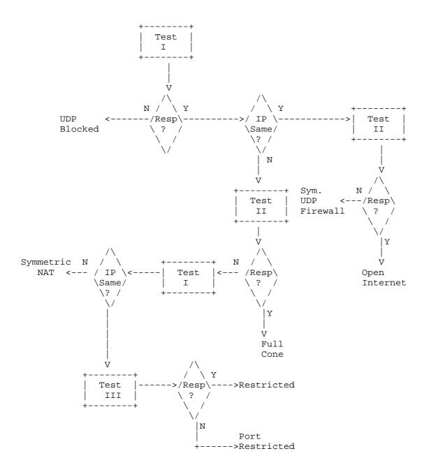
Figure 2: Flow for type discovery process
